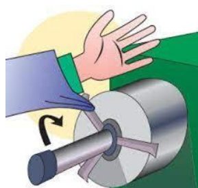
Entanglement: with a moving protruding part
