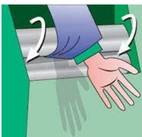
Catching: two rollers rotating in opposite directions
