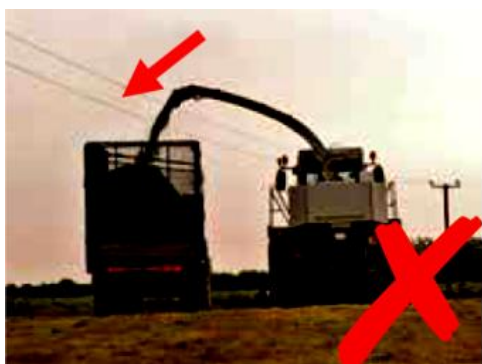
Non isolated electric cables
