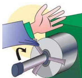
Entanglement: with a moving protruding part
