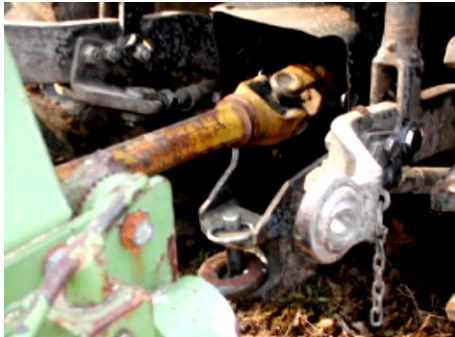
Unprotected cardan shaft
