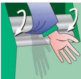
Catching: two rollers rotating in opposite directions
